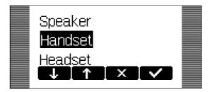
Here, the volume of the casing speaker, handset speaker, or headset speaker can be adjusted. Select one of the three choices.
